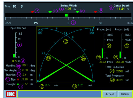
Figure 3: the cross-point of the needles - representing mixture velocity and mixture density - indicates mixture production
